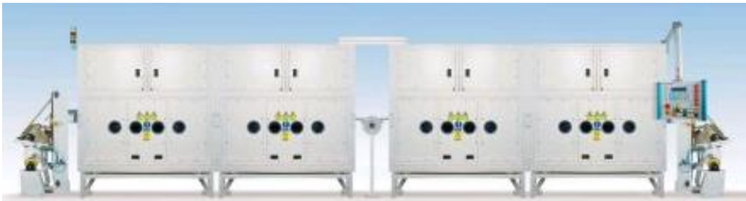
Figure 2. NS-Line (four units) for mass production of nanofibers [10]
