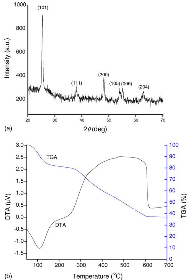
Fig. 1. (a) XRD pattern of heat-treated  $\text{TiO}_2$  (anatase phase) nanofibers after calcination and (b) TGA/DTA curves (10 °C/min ramp rate).
