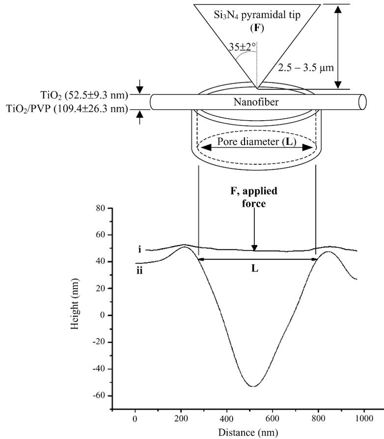
Fig. 3. (a) Schematic diagram of three-point bending test and (b) actual AFM scanning data on fiber (i) and pore (ii).
