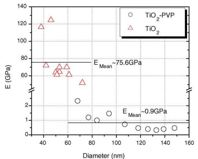
Fig. 5. Young's modulus ( $E$ ) vs. diameter of TiO<sub>2</sub>-PVP and TiO<sub>2</sub> nanofibers.
