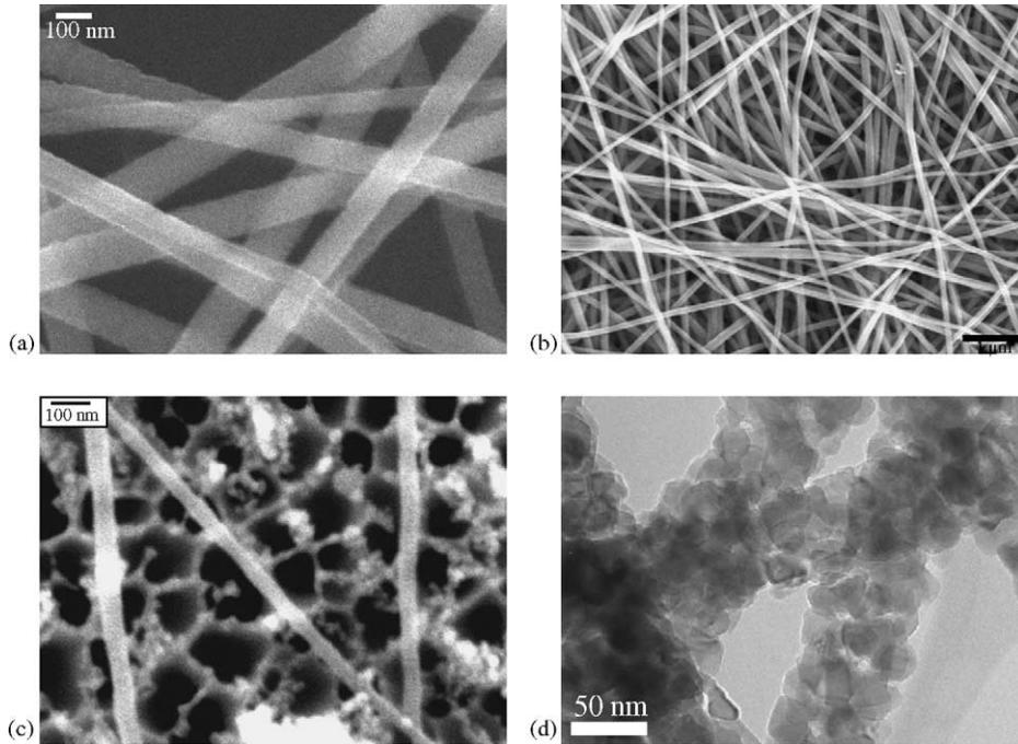
Fig. 2. SEM images of (a) TiO<sub>2</sub>/PVP nanofibers, (b) TiO<sub>2</sub> nanofibers, (c) TiO<sub>2</sub> nanofibers suspended over pores of Al<sub>2</sub>O<sub>3</sub> membrane, and (d) TEM image of TiO<sub>2</sub> nanofibers.
