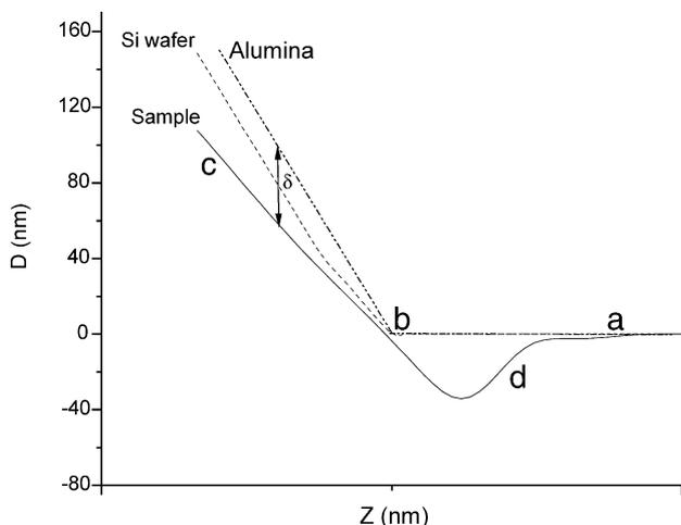
Fig. 4. Examples of cantilever deflection ( $D$ ) vs. sample height curves ( $Z$ ).
