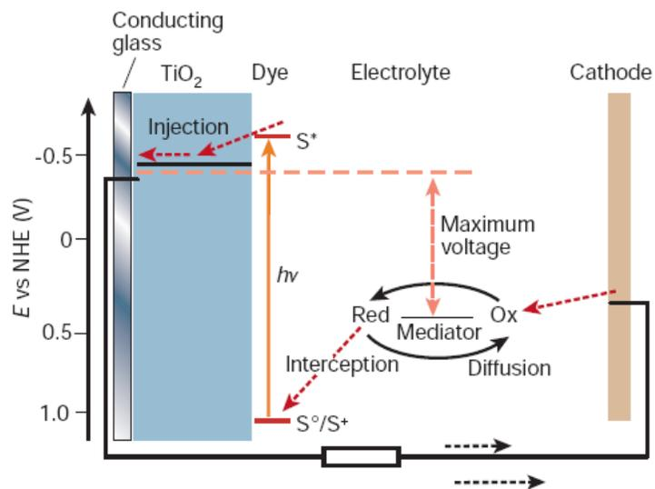
**Figure 4.** Schematic illustration of dye-sensitized solar cell.
