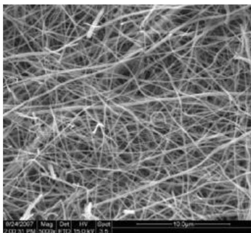
**Figure 5.** TiO<sub>2</sub> nanofiber produced by Nanospider™ technology (Copyright © 2009 Elmarco)
