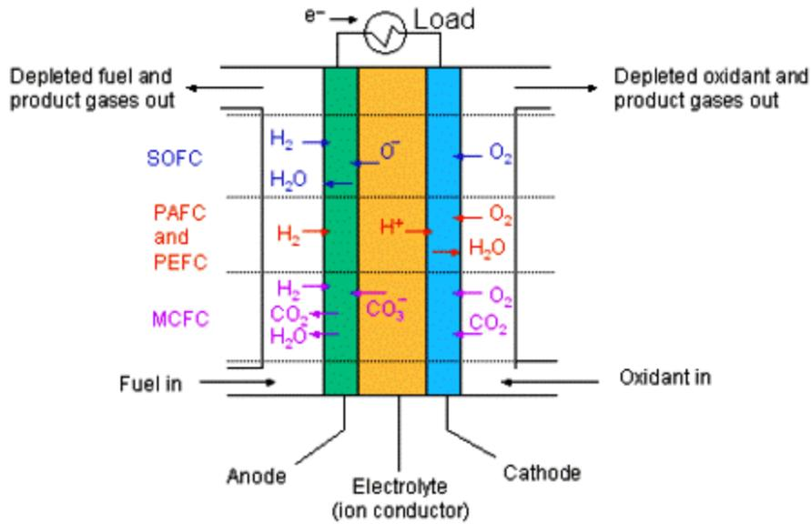
**Figure 2.** The five principal types of fuel cells and their electrochemical reactions [5]
