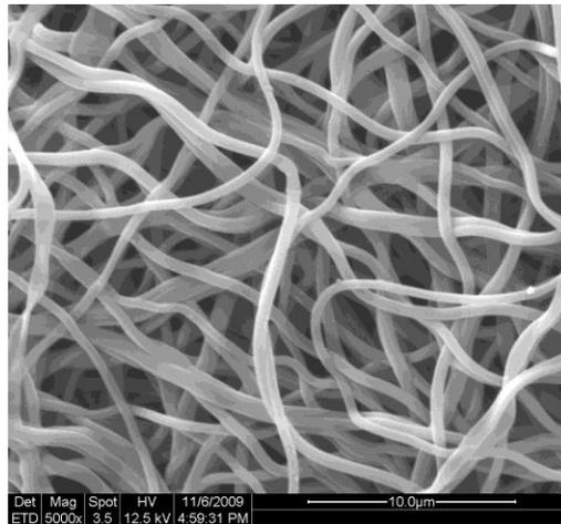
**Figure 3.** PAN-based carbon nanofiber produced by Nanospider™ technology (Copyright © 2009 Elmarco)
