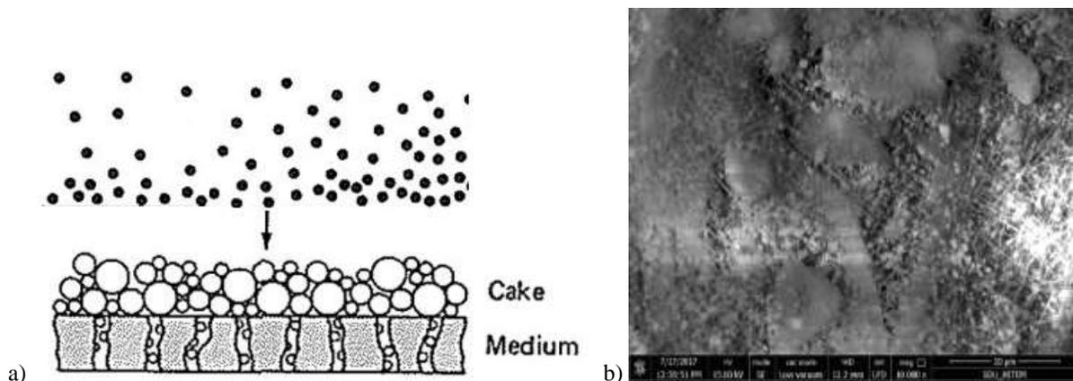
Figure 3. a) Cake filtration, b) Deposition of the particles on the upper side of the nanofiber media
