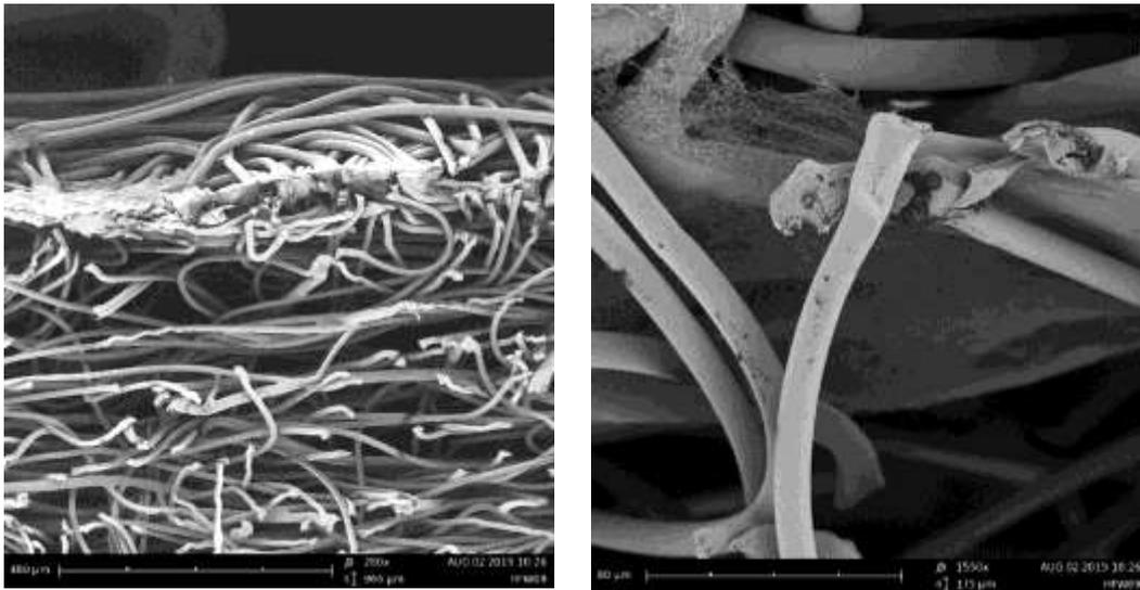
Figure 4. Cross-section of composite filter including nanofiber inter layer a) Magnification of 280x and b) 1550x
