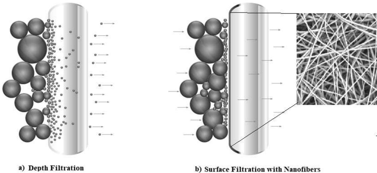
Figure 2. a) Depth filtration, b) Surface filtration with nanofibers
