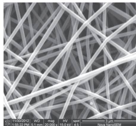
**Figure 3.** SEM picture of PAN nanofibers
