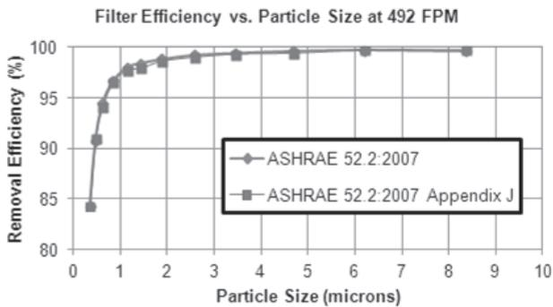
Figure 4. Effect of discharge on filtration efficiency
