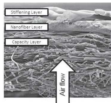
**Figure 1.** Cross-section SEM picture of the composite media
