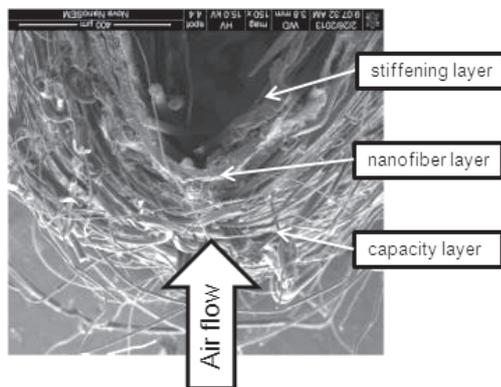
Figure 5. SEM picture of a pleat-tip of composite media
