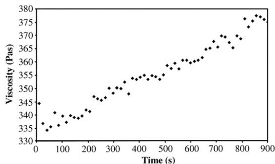
Fig. 2. Viscosity of the prepared sol used to prepare TiO<sub>2</sub> nanofibers.
