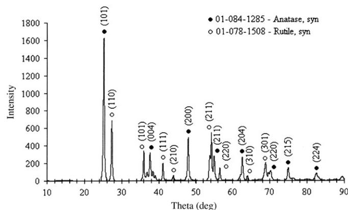
Fig. 3. XRD result of the prepared TiO<sub>2</sub> nanofibers.
