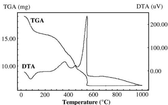
Fig. 1. DTA/TG analyze of the prepared sol used to prepare TiO<sub>2</sub> nanofibers.
