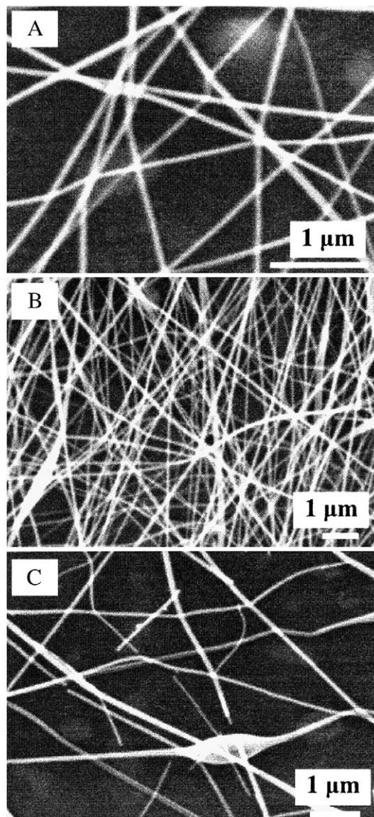
Fig. 4. SEM images of TiO<sub>2</sub> nanofibers prepared at A) 1, B) 1.25 and C) 2 kV/cm of electric field.
